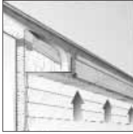
Figure 5.4 Continuous Soffit Vent
